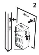
Stick the sampler to a vertical surface where it will not be disturbed or touched such as a wall, pillar or rack. Can also be mounted inside racks, cabinets and air ducts.
